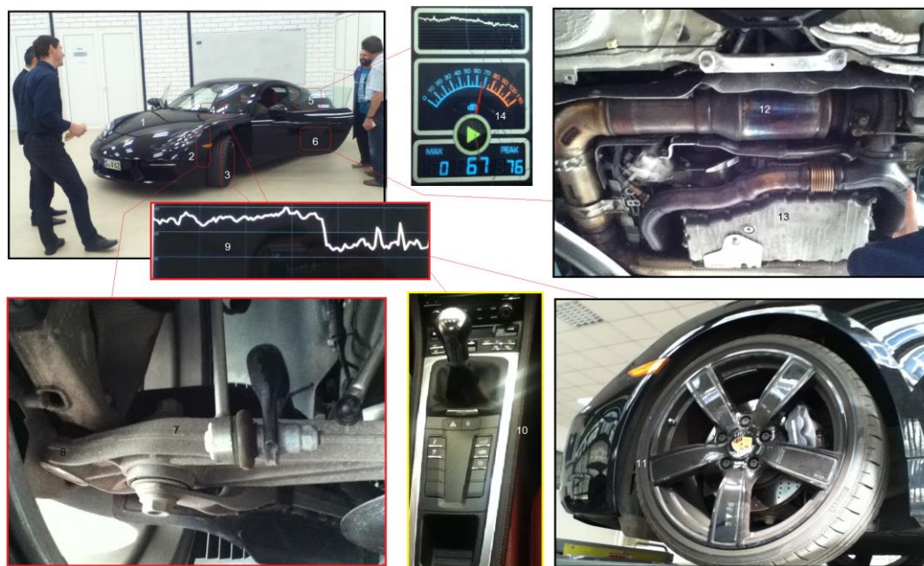
Figure 7. Research equipment from Technical University and studied Porsche Cayman. 1-Tested car; 2-front suspension; 3-wheels; 4-on-board recording equipment; 5-engine sound measurement; 6-power train; 7-lower suspension arm; 8-joint; 9-sound curve; 10-gear change; 11-tire; 12-exhaust; 13-gearbox; 15-software app.
