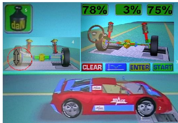
Figure 4. Schematic image of vehicle on vibrational test bed.
