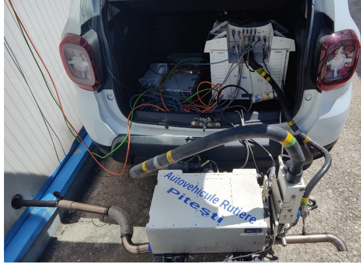
Figure 8. Portable Emission Measurement System connected to the ETB
