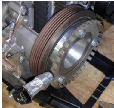
Figure 4. The setup for the crankshaft position measurement
