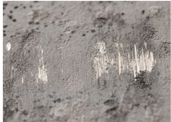
Figure 5. Surface of the sample after applying the wear cycles
