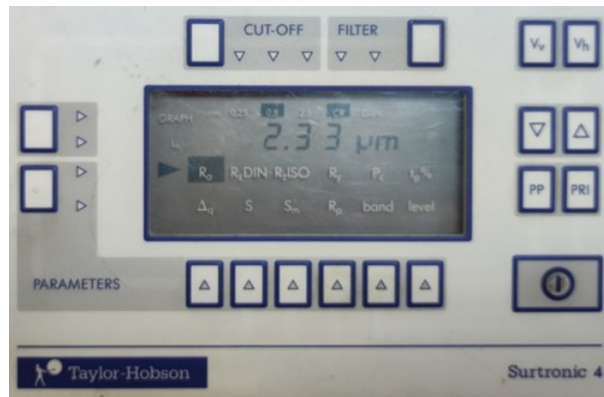
Figure 3. Surface roughness measurement of the sample
