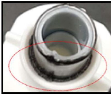
Figure 8. Excess material resulting from the welding process
