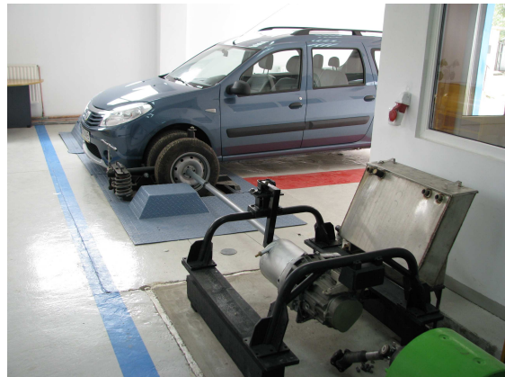
Figure 12: The test bench for hybrid electric and electric vehicle under construction in the Alternative Propulsion System & Renewable Energies laboratory , Automotive Engineering Research Centre, University of Pitesti
