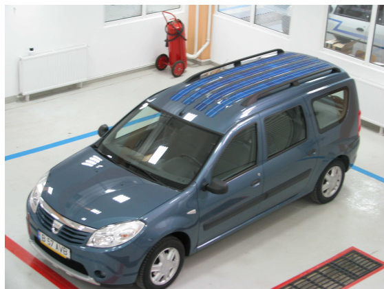
Figure 8: GRAND SANDERO HYBRID with photovoltaic cells placed on the roof
