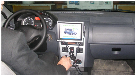
Figure 9: Multitasking display used to illustrate the energy flows in the EcoMatic Hybrid System
