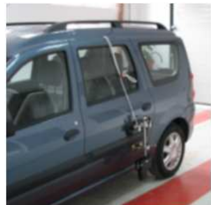
Figure 13: The DATRON CORREVIT equipment for measuring the dynamic performances of the vehicle on the road
