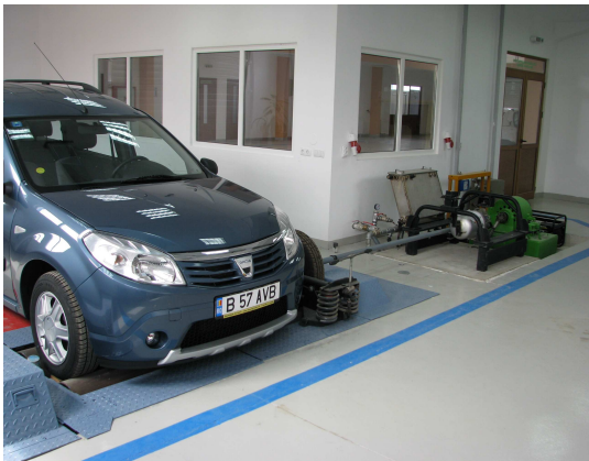
Figure 12: The test bench for hybrid electric and electric vehicle under construction in the Alternative Propulsion System & Renewable Energies laboratory , Automotive Engineering Research Centre, University of Pitesti
