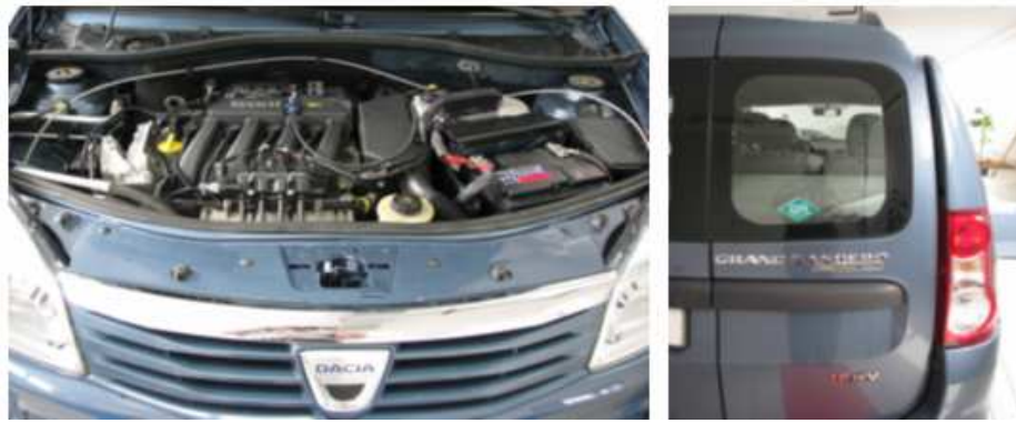
Figure 5: DACIA GRAND SANDERO HYBRID LPG -electricity with Renault K4M-690 1,6 liters-16V engine fuelled with LPG by Landi Renzo OMEGAS installation
