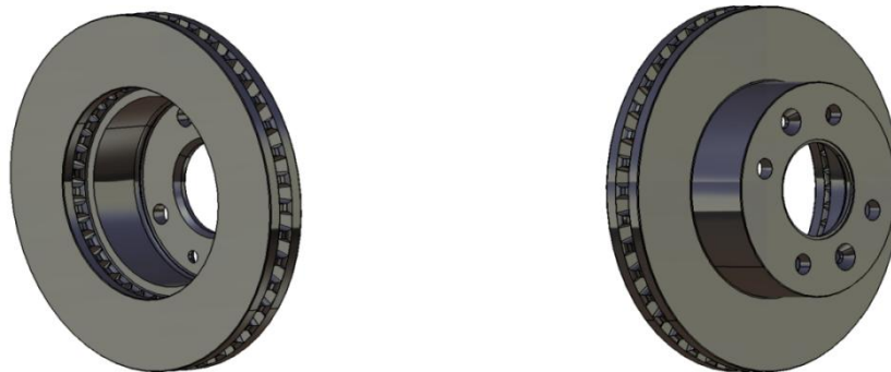
Figure 1. The 3D model of the brake disc analysed.
