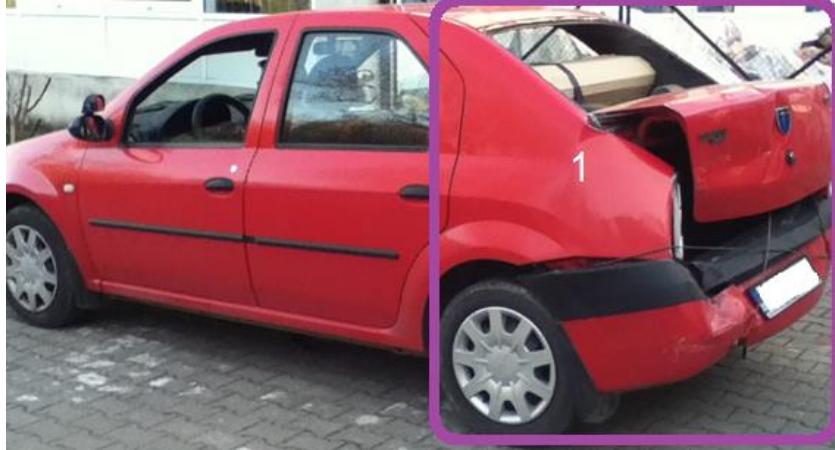
Figure 2. Vehicle after the road-traffic event. 1-crashed area.
